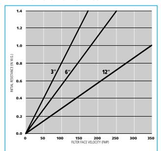
NOTE: This graph represents a typical rating. 3 & 6" filters are tested at 100 FPM and 12" filters are tested at 250 FPM at the factory. The inside face dimension (not including filter frame) is used to calculate resistance. Recommended service restriction is approximately two times the initial restriction at the factory test flow rate.
